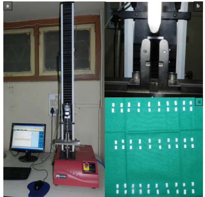
[Table/Fig-6]: a) Instron universal testing machine; b) Three point bend test for flexural strength testing; c) Samples after testing.
